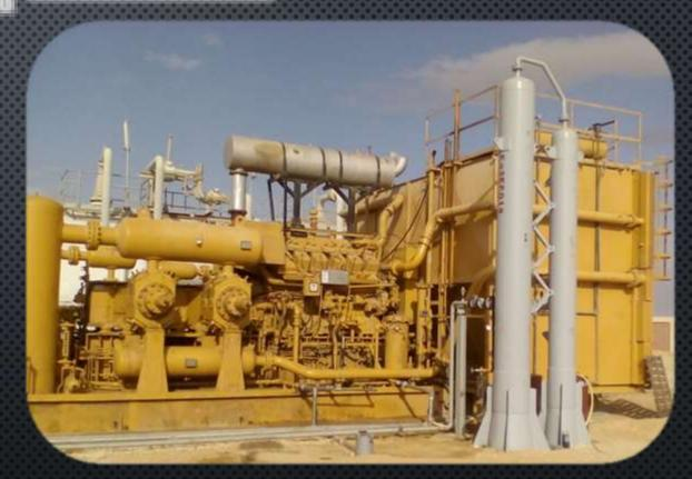
RENTAL OF ARIEL GAS COMPRESSION PACKAGE FOR GAS LIFT DELIVERING 8 MMSCFD FROM 150 PSI SUCTION PRESSURE TO 1800 PSI DISCHARGE PRESSURE.
