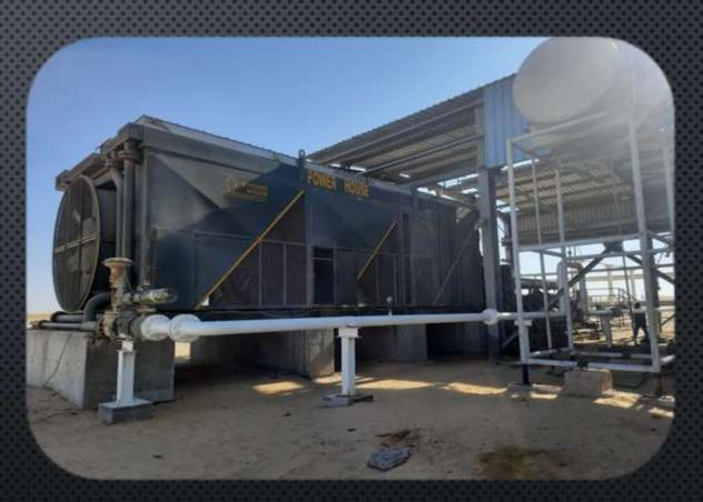
RENTAL OF BOOSTER GAS COMPRESSOR TO BOOST 5 MMSCFD GAS FROM 1.5 BAR SUCTION PRESSURE TO 68 BAR DISCHARGE PRESSURE.
